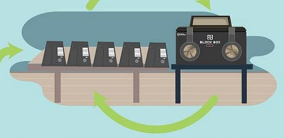
BlockBox Lab Forensic tools require nteraction with a device, for example to install bootloaders for password cracking. After this initial phase, devices can be placed in shielding bags to free up the box.
