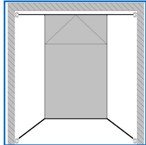
4. The installation should start at the bed head by drawing the cable rope through the thread eyes of the canopy. Now start slowly to strain the rope until the ropes is energized and don't sag.
